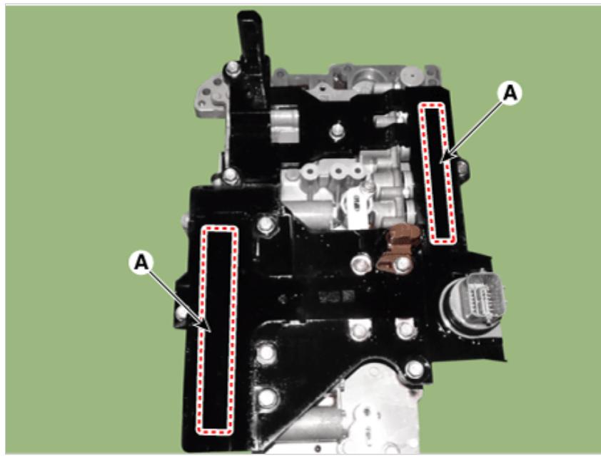
7. Remove the solenoid valve support bracket (A).
