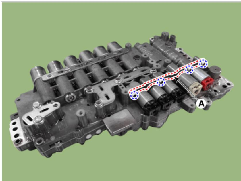
8. Remove the damper clutch control solenoid valve (A).
